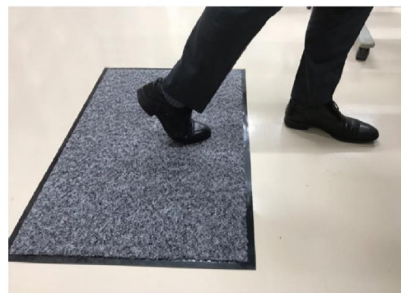
The sensor communicates wirelessly to a PC using electricity generated when a person passes by
