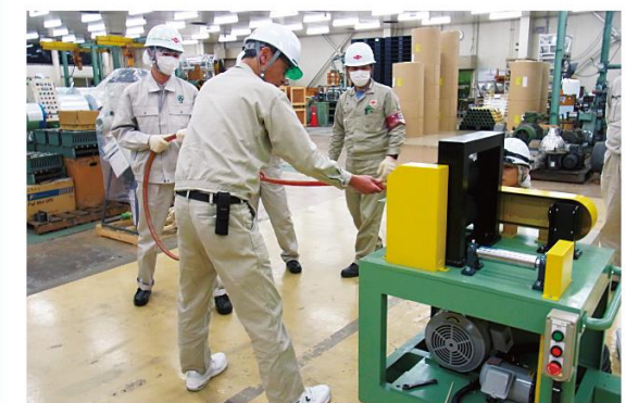
Simulation of a rubber hose being caught in a rotating object
