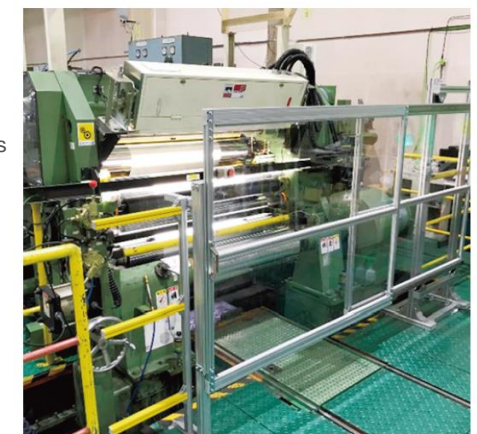
Entry prevented by installing covers all around the production facility
