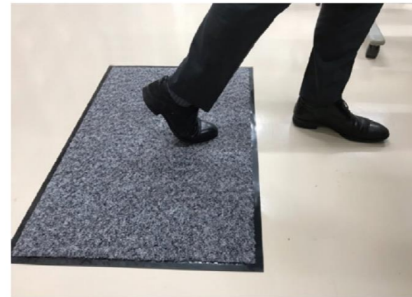
The sensor communicates wirelessly to a PC using electricity generated when a person passes by
