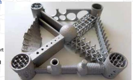
A part manufactured by aluminium alloy powder 3D printing
