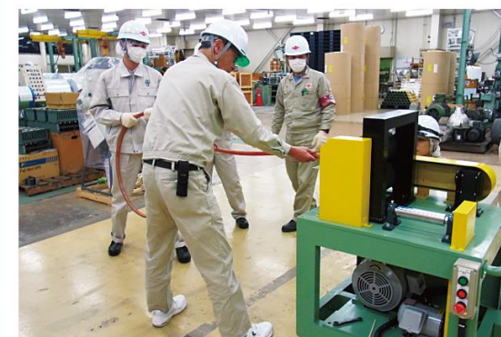
Simulation of a rubber hose being caught in a rotating object
