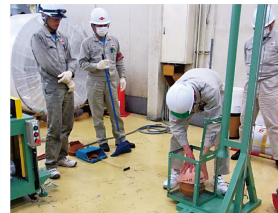
Simulation of falling shock absorption with and without a helmet
