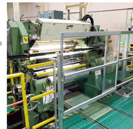
Entry prevented by installing covers all around the production facility
