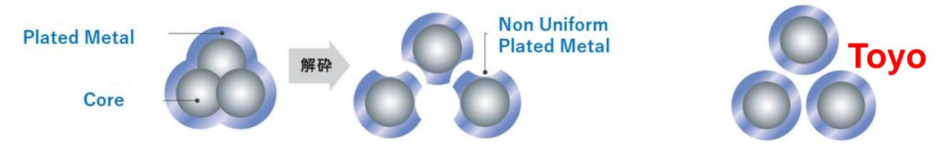
Nano-size dispersed plating also possible in order to enhanced characteristics of both the plated metal and core particle. Doublelayer functional plating with different metals, such as, for example, creating the outer contact layer and the middle layer as buffer/barrier over the core particle.
