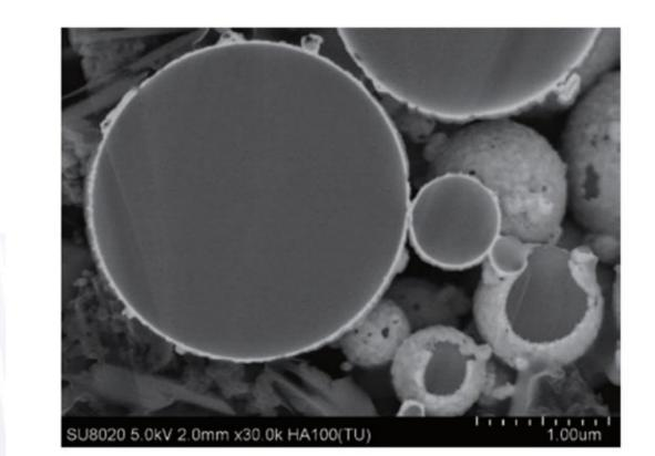
The Ag-coated AI and Cu particles helped in reducing the amount of metallization laydown due to the volume/weight balance
