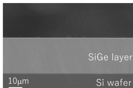
Fig.2 SEM cross-section of SiGe/Si wafer.
