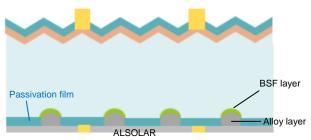
Fig. 2; Structure of PERC solar cell
