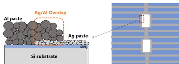
**Fig. 2** Cross sectional images of Al/Ag interface
