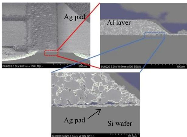
**Fig. 5** Cross sectional SEM images of Ag/Al interface by using Pb free GF
