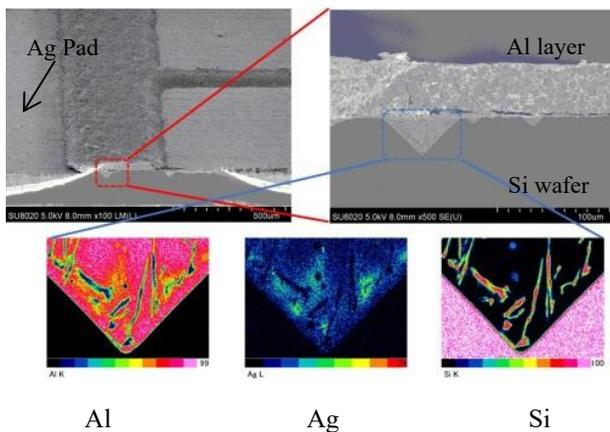
**Fig. 4** Cross sectional SEM and EDS images of Ag/Al interface by using Pb GF
